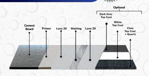
Enhance your Cement Board Roof with Lava 20 Waterproofing System for unmatched adhesion. Unlike traditional coatings, polyurethane forms a strong bond with the smooth, non-porous surface. This liquid coating penetrates and fills cracks and gaps, creating a durable, peel-resistant seal. Waterproof your roof against damage, ensuring longevity and performance.
